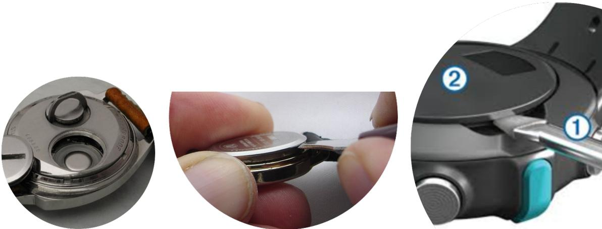
Clip fastening without screw, no tool required, and clip fastenings secured with glue, may require some form of tool. Would gluing acceptable as a non-replaceable closure?
